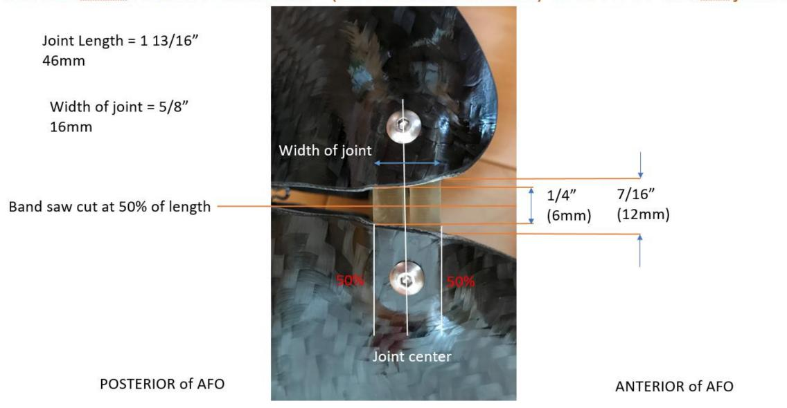
50% less Dorsi-Flexion Joint Return - Open Anterior (versus Max Return cut) Good for Standard joint or free DF joint Joint Length = 1 13/16" 46mm Width of joint = 5/8" 16mm Width of joint 3/4" † 5/16" Band saw cut at 50% of length (19mm) (8mm) 13/16" (20mm) **POSTERIOR of AFO** Joint center **ANTERIOR of AFO**
